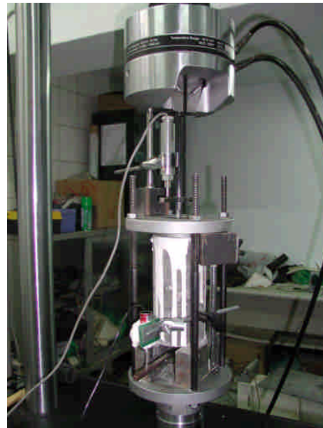
Fig. 4. The set-up of pullout test
