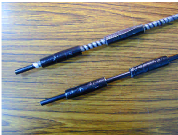
Fig.3. The PVC sleeves of the GFRP rebars
