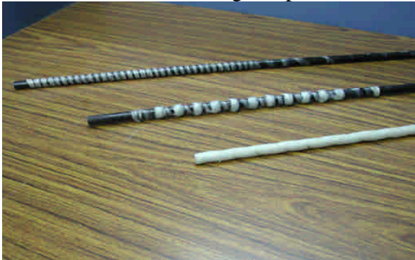
Fig. 1. GFRP rebars made from different winding methods (top: beta, bottom: Aslan)
