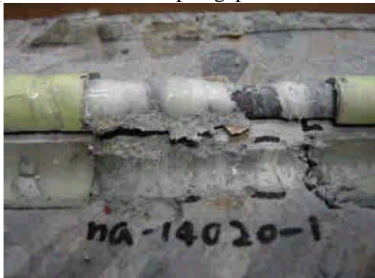
Fig. 10. Failure mode of a transverse/no axial wound specimen
