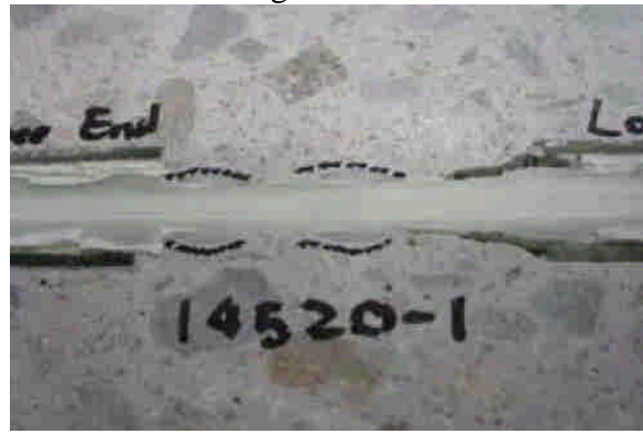
Fig. 11. Failure mode of a helical/axial wound specimen
